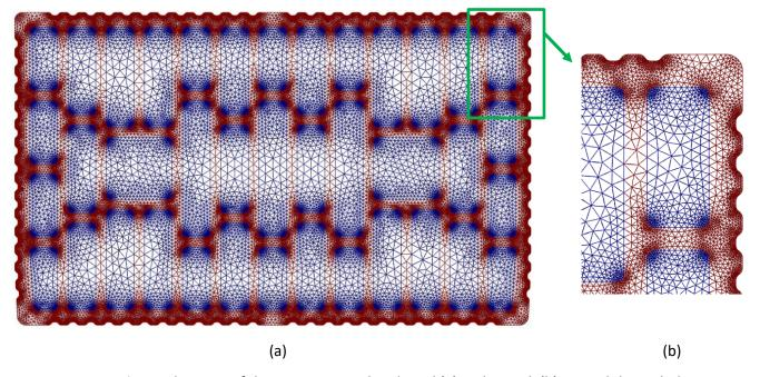
Fig.2. Schematic of the computational grid used (a) in the Brick (b) around the air hole.
