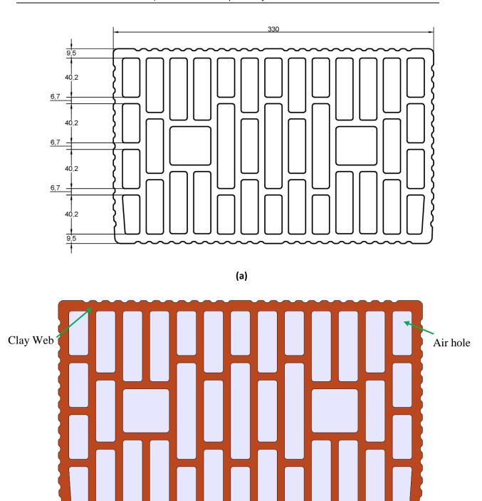
Fig. 1. (a) Brick geometry dimensions in mm and (b) domains of porous clay and air holes.
